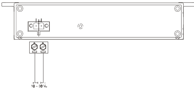
Figure 2-20 Power Connection for EDG-4504
